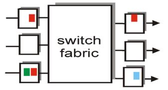
output port contention at time t - only one red packet can be transferred
