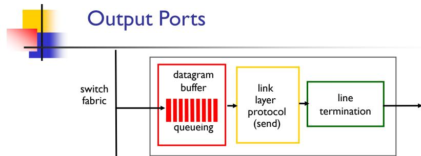
buffering required when datagrams arrive from fabric faster than the transmission rate
